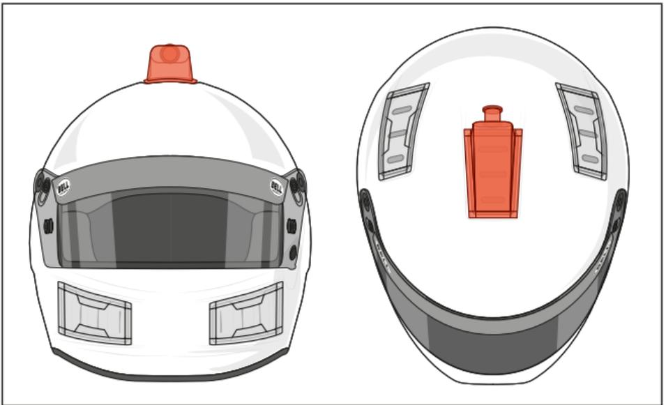
Before installing the Forced Air insert, remove the protective cover from the back side of the Forced Air insert exposing the adhesive material that will seal the Forced Air insert to the helmet shell. Once installed press firmly around the edges of the Forced Air insert to assure proper adhesion.
