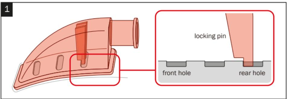
Place the Forced Air and Cover Plate Seal on top of the Forced Air insert to ensure a perfect seal and prevent air from entering.
